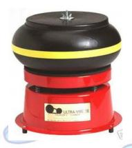
The buttons are vibrated in the machine, along with ground walnut hull media. (Ground corn cobs can also be used, but I have been told that they need to be replaced more frequently than the walnut shells.)
